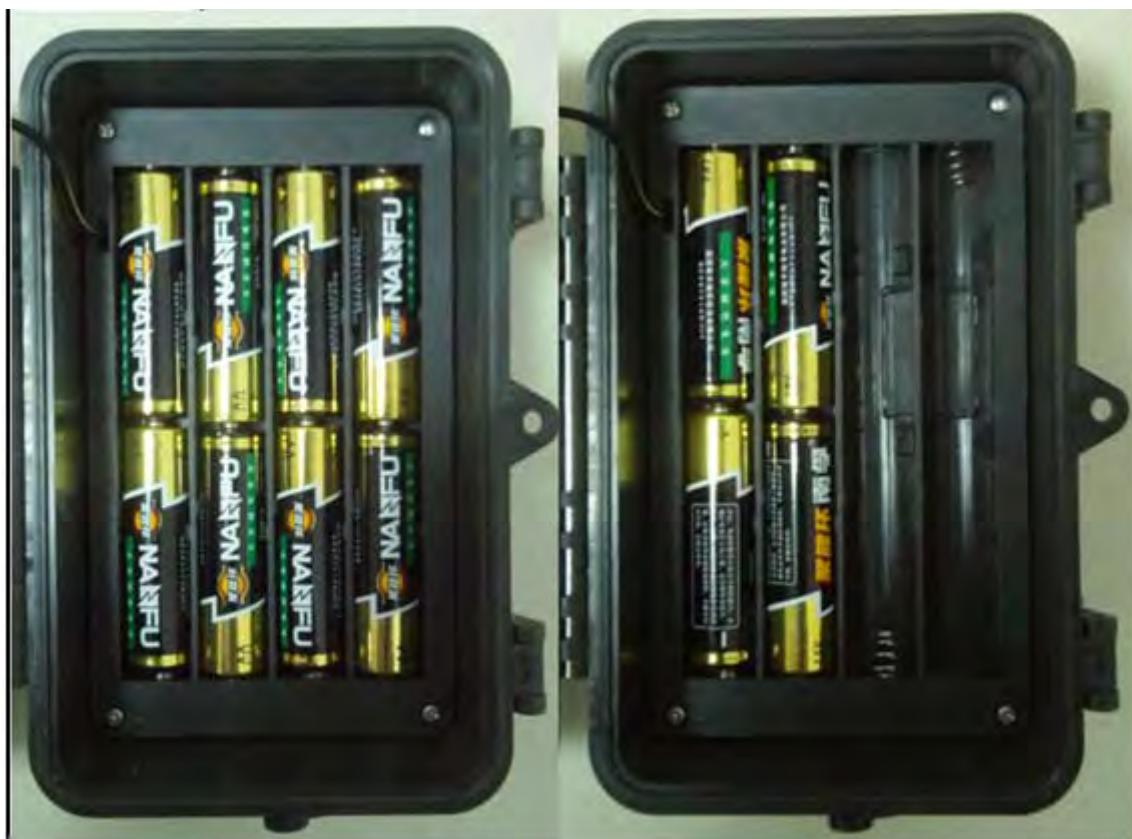
Fig. 5: Battery Configurations of 8 or 4 batteries
