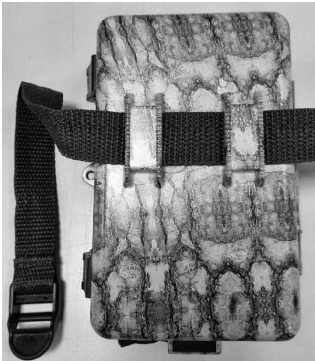
Fig 7: Fixing the camera with belt Using bottom screw.
