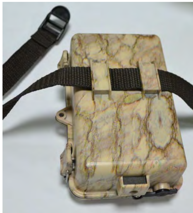
Fig. 7: Fixing the camera with belt Using bottom screw
